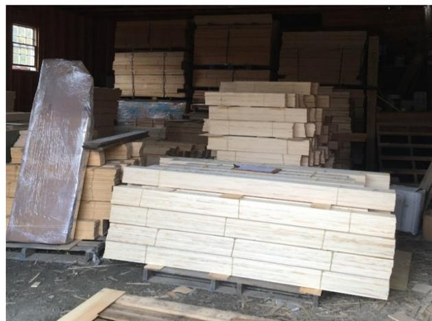
Mill director **Robert Tanner** visited Ward Clapboard Mill, Moretown, Vermont, where the siding is being prepared. A mill site in operation since 1868, **Ward Clapboard Mill** turns whole logs on a lathe, then uses an indexing and sawing mechanism to cut clapboards
